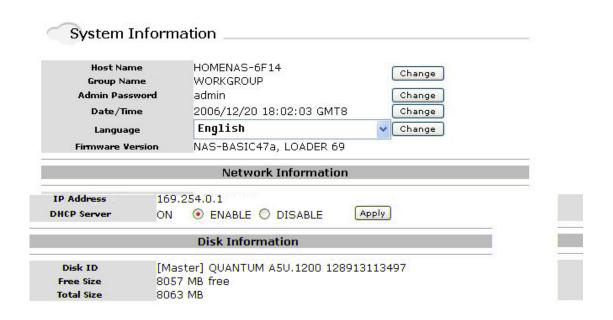
The welcome screen displays the IP address, firmware version and the hard drive information such as the hard drive type and storage space available.
